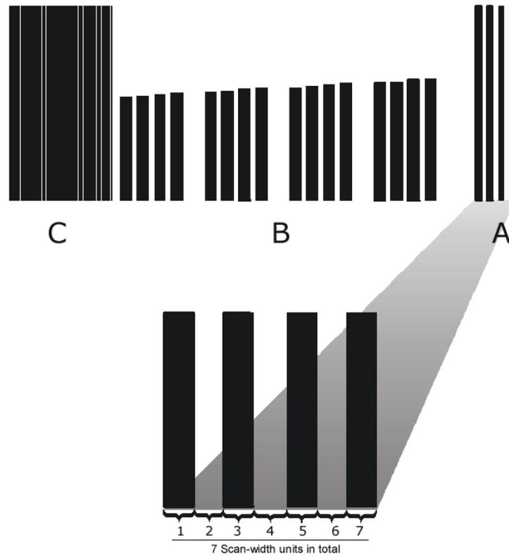
The **A** part of the pattern consists of scan-width units (SWU).
