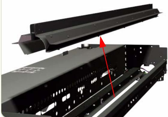
10. Remove the Reflector Assembly from the scanner.
