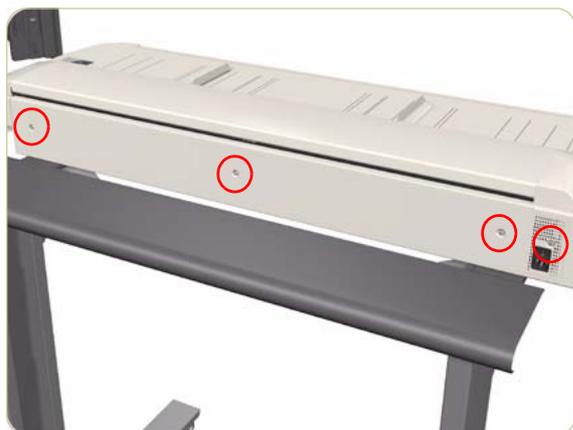
1. Remove 4 screws that secure the Rear Cover to the rear of the scanner.
