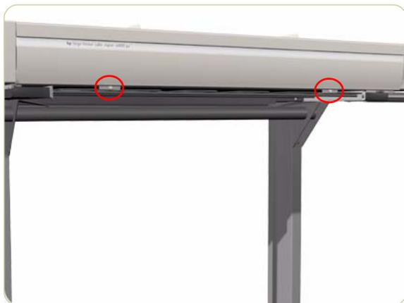
1. Remove the 2 screws along the lower edge of the Top Profile.
