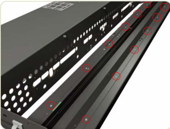
9. Remove 12 screws from the Reflector Assembly.
