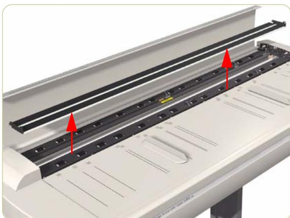
3. Carefully lift up the Glass Plate and remove from the scanner.
