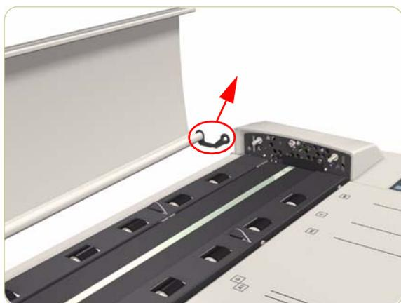
4. Remove the Top Profile from the scanner.
