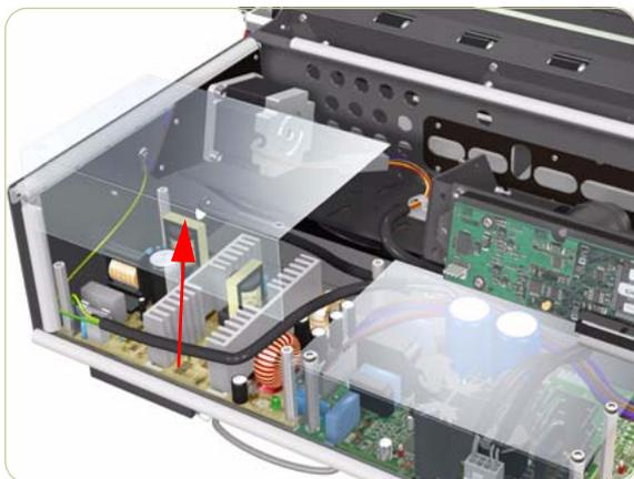
6. Remove the 4 screws that secure the Power Supply Unit.
