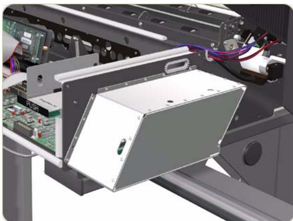
4. Pull out the Interface Board Cover slightly and disconnect the cable that is connected to the Interface Board from inside.
