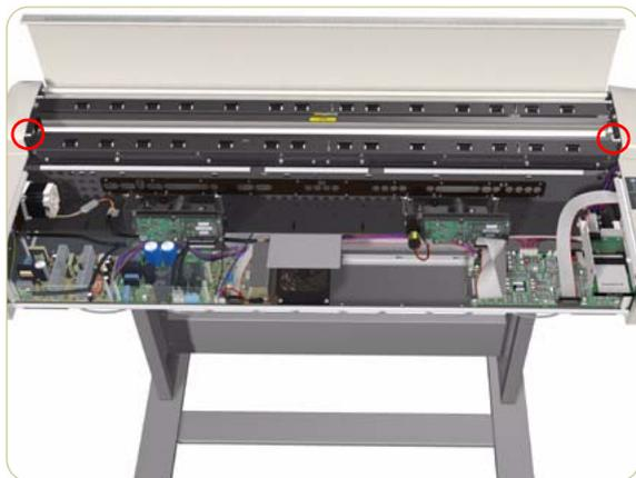
5. Loosen 16 screws on the front side of the Entry Roller Shield.
