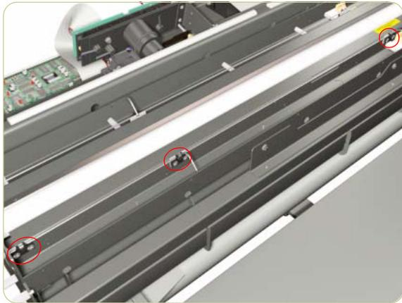
**11.** Loosen the screws from the bearings that secure the Media Detector Wires.
