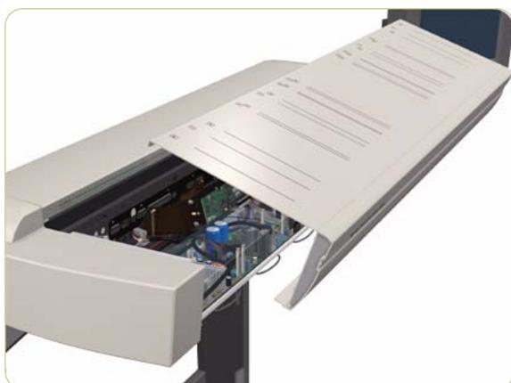
3. Lift up the Top Cover and remove from the scanner.
