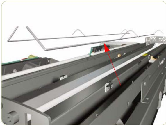
**12.** Remove the Media Detector Wires from the scanner.
