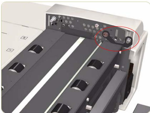
6. Loosen 16 screws on the rear side of the Exit Roller Shield.
