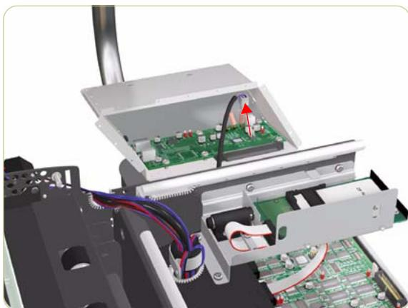
5. Remove the Interface Board Cover from the scanner.
