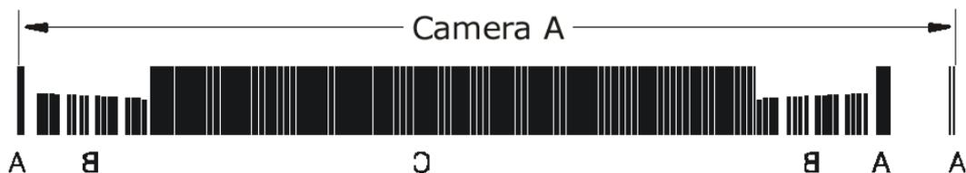
Camera A scans from right to left, so the image above is a mirrored section of the total **Scan-Width pattern** as the copier actually sees it. The camera only sees a single line of pixels with the green CCD pixel line that
