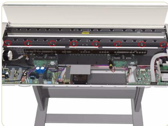
6. Gently remove the Entry Roller Shield from the scanner. Be careful NOT to bend it or damage it while removing.
