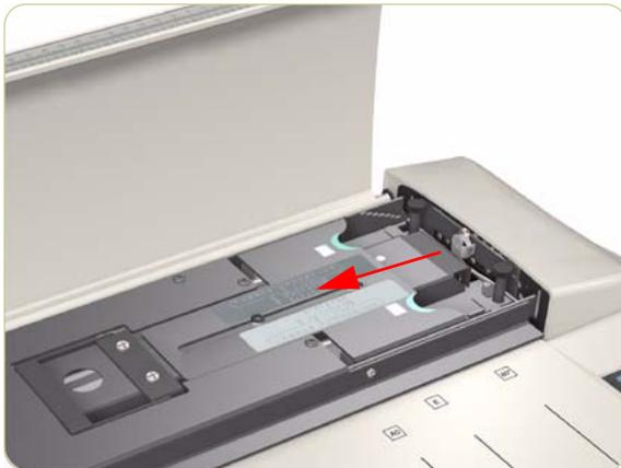
**2.** Release the lock on both sides of the Guide Plate.
