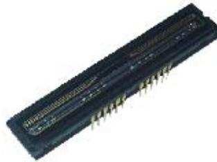
The CCD is formed as a chip, and is inserted into a standard dual in-line socket just like a normal chip. The chip has 3 rows each containing 10000 pixels.
