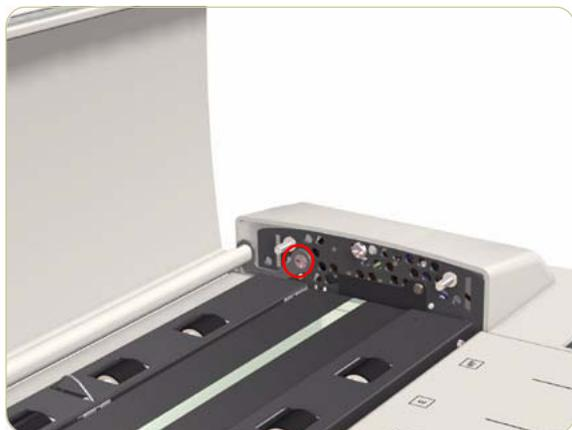
3. Slide the bearing out of the pivot in the Top Profile.
