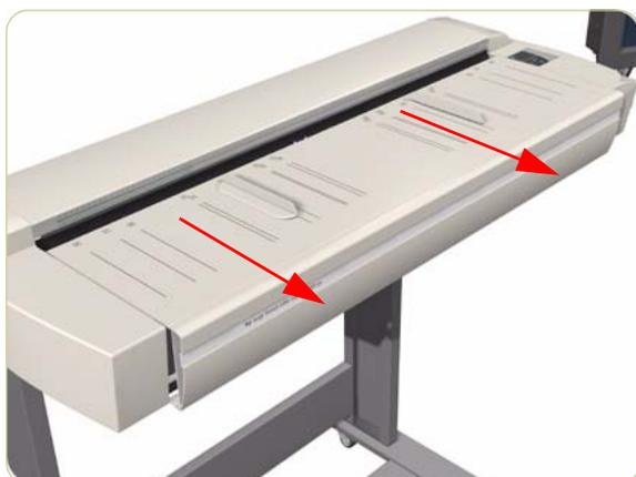
2. Pull the front part of the Top Cover away from the scanner in order to release the upper part of the Top Cover.
