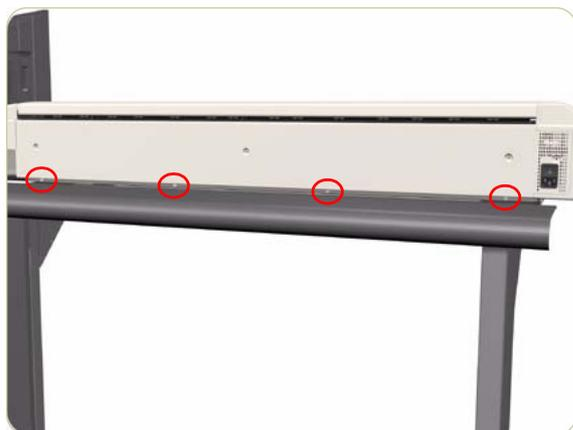
2. Remove 4 screws that secure the Rear Cover to the lower edge of the scanner.
