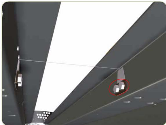
4. Install the second Leaf Spring using 2 screws, making sure the wire is continuously tensioned.
